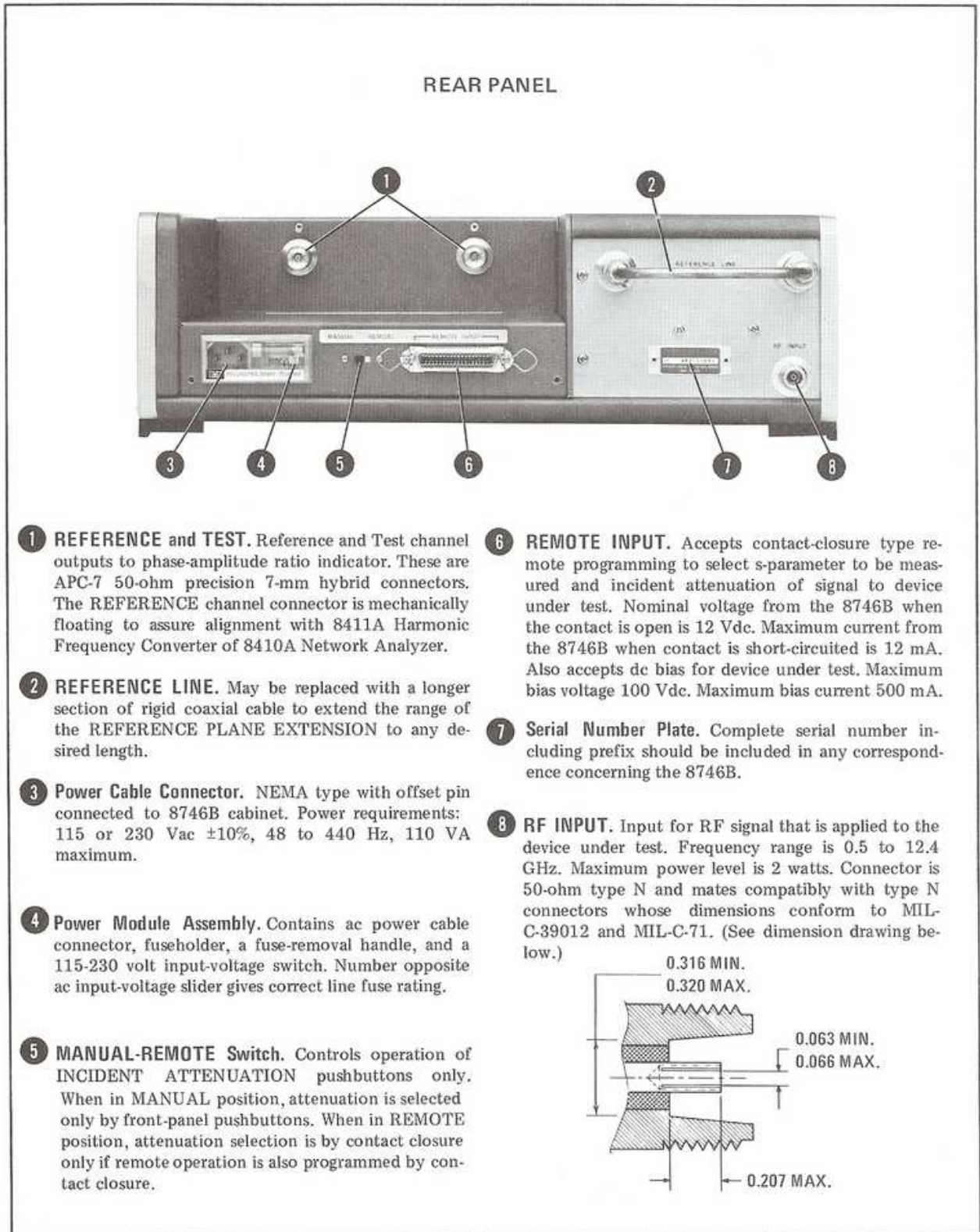
Figure 3-3. Rear Panel Features
